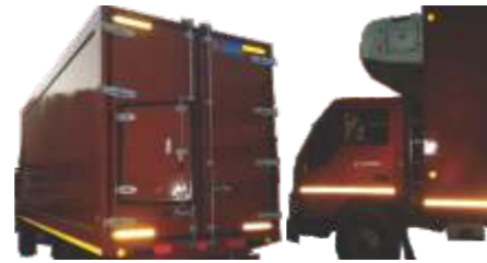
Radium Line : Front side, back side yellow reflection radium line for night time.
