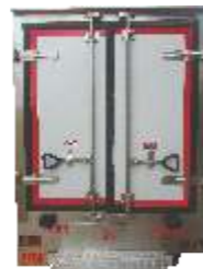
Door Frame : Door frame "C" Profile having 2mm SS Sheet.
