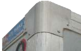
Bucket Structure: Design on bended Aluminium panel with 4 mm thickness & SS Corner Profile for solid covering of container.
